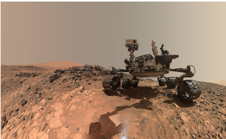
This low-angle self-portrait of NASA's Curiosity Mars rover shows the vehicle at the site from which it reached down to drill into a rock target called "Buckskin" on lower Mount Sharp.
