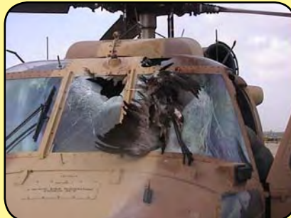
Damage to military helicopter from crane strike. Photo courtesy of Dept. of Defense
