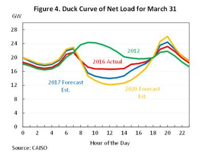
The actual net load on March 31, 2016 shows just the beginning of a duck curve. The lowest net load is in the middle of the day when the sun is shining, and there is a relatively steep ramp-up in the evening to meet the peak evening load. There is also a notable smaller peak in the morning while the sun is still low in the sky but activity has already begun for the day.
