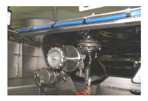
External piping on a DOT407 or MC307 tends to be short (less than two feet) and can be at either rear or at side of trailer, depending on style of loading and unloading.
