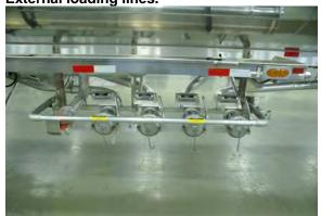
DOT 406: 1 compartment – 1 wetline and 1 Line used for vapor recovery
