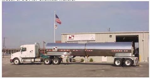
Flammable liquids chemicals and solvents also are hauled in cargo tanks. The most common type tank for these products is the MC307 or DOT407 with capacities of from 5,000 to 7,000 gallons.
