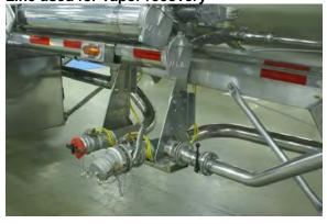
Flammable liquids such as gasoline and diesel fuel also are transported in straight trucks where the tank sits on the truck chassis. The capacity of these tanks ranges from 1,500 to 4,500 gallons. The external piping is much shorter on these tanks and will hold less product.
