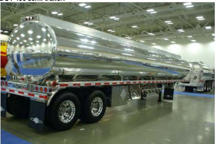
Typically up to 9,000 gallon capacity with four to five compartments to allow transportation of different grades of gasoline or petroleum products.
