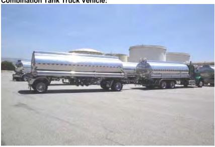
This is a typical truck and trailer combination which is commonly used on the West Coast. The external piping on the pull or pup trailer is more exposed than the piping on the truck mounted tank.
