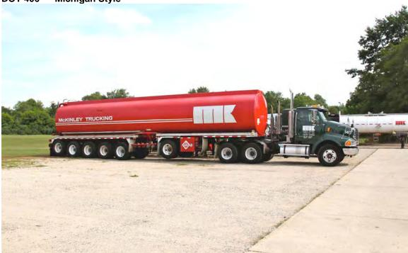
This Michigan style DOT406 trailer can haul up to 12,000 gallons, because of the extra axles. The axles provide a protective barrier making it even more unlikely that wetlines could be damaged in an accident.
