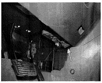
Virtually every passenger car and light truck manufactured in or imported to the North American market since model year 1996 includes an Environmental Protection Agency (EPA) mandated DLC to allow access to engine and emissions diagnostic data.
