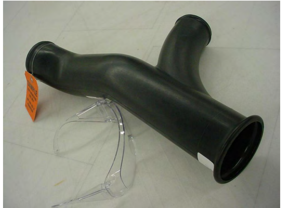
Injection Molded Nylon Part: Example part weight ~2 lbs DecaBDE content ~41 grams (<5% by wt)
