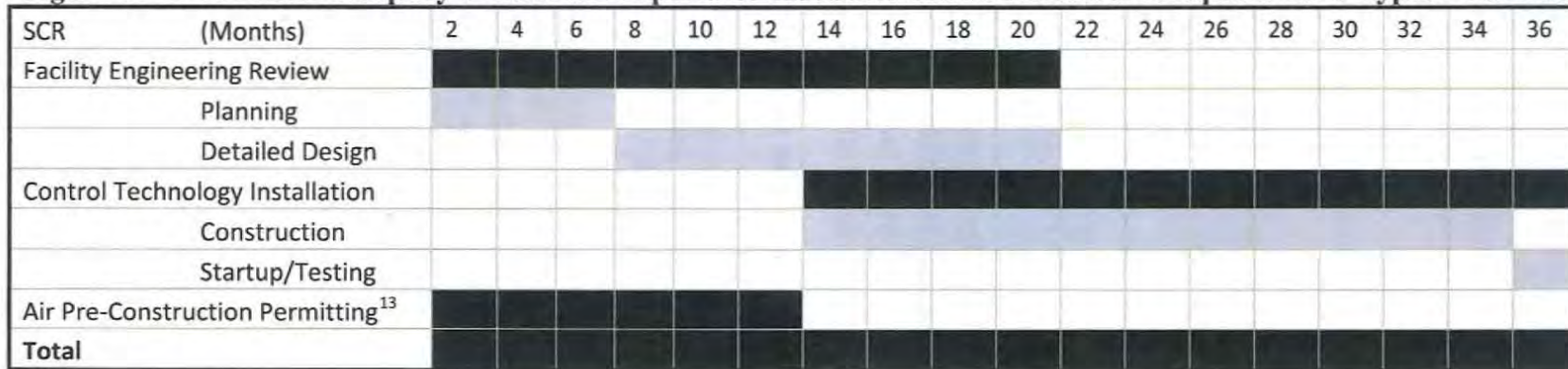
Figure VI-1. Southern Company's Historical Experience Illustrates that 36 Months are Required for a Typical SCR Installation
