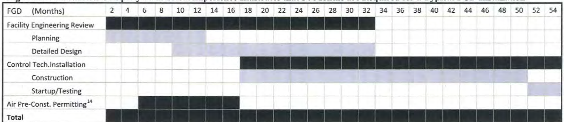
Figure VI-2. Southern Company's Historical Experience Illustrates that 54 Months are Required for a Typical FGD Installation
