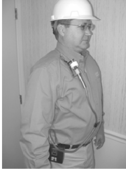
FIGURE 3-1—RESPIRABLE DUST SAMPLING SETUP
