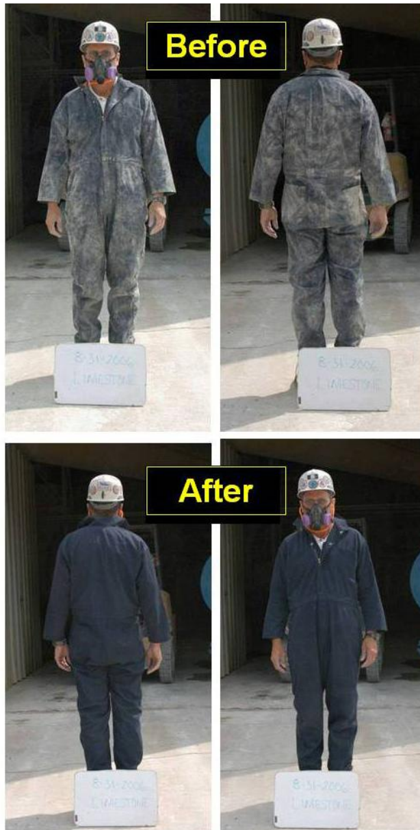
Figure 8.3. Test subject wearing polyester/cotton blend coveralls before and after using the clothes cleaning booth.
