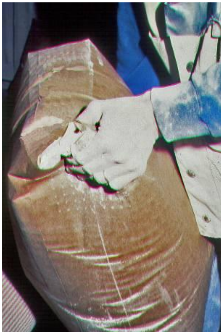
Figure 8.11. Worker closing bag valve with his hand as he removes the bag from the fill nozzle, significantly reducing his dust exposure.
