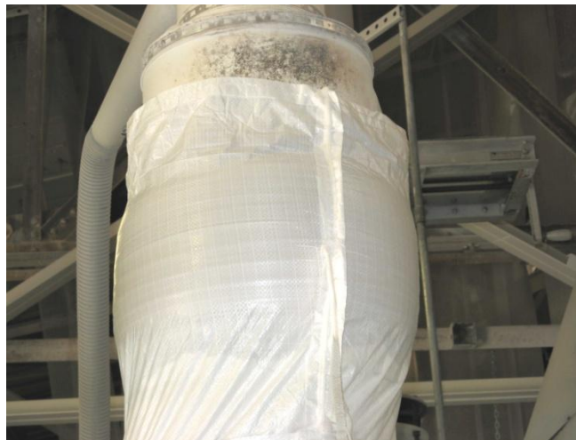
Figure 6.20. Expandable neoprene rubber bladder used in the fill spout of the bagging unit for Flexible Intermediate Bulk Containers.
