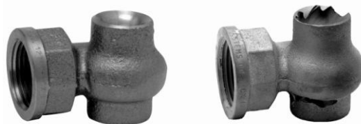
Figure 2.15. Nozzle erosion—new versus used [Schick 2006].
