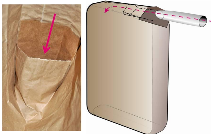
Figure 6.2. Typical bag valve—interior view (left). Artist concept of fill nozzle and bag valve (right). Fill nozzle enters through the bag valve and delivers product into bag.
