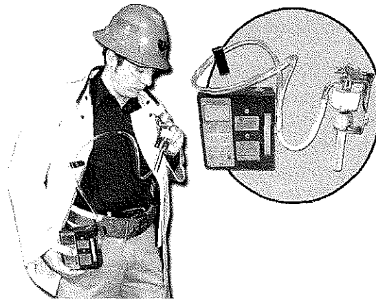
Figure 2-5 Respirable Dust Sampling Setup
