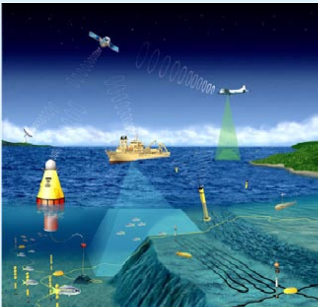
Ocean observing systems link data collected from multiple platforms such as ships and in-situ monitoring stations with remote sensing capabilities from satellites, submersibles and aircrafts. Source: Ocean.US
