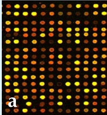
a) Microarrays contain microscopic spots of DNA samples with each spot representing a different gene. The intensity of dye in each spot is used to quantify the expression of each gene in a sample, for example in seawater. (b) The BreveBuster is a submersible device that assesses the presence of a red tide by identifying and counting Karenia brevis . Photo credit: a. D. Crawford, b. G. Kilpatrick
